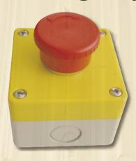
Emergency stop button mounted on a thermoplastic or aluminium alloy housing with IP65 protection. It can also be ordered without housing for front panel assembly. The button is available as a momentary or latching mechanism, which can be released by twisting or pulling. The NC circuit is designed as a positive break operation. Up to two switching modules (either NC or NO ) in any combination can be mounted to the button unit. Housing is available as a grey, yellow or sandblasted finishing.
